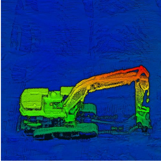
LIDAR image taken from RTL-400; altitude 100 ft, speed 13 mph
