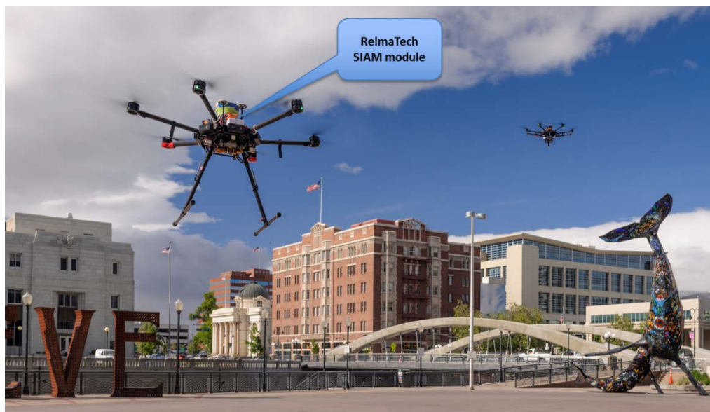
UAS fitted with a RelmaTech SIAM module (small white box), NIAS-NASA UTM TCL4 Operations, Reno Plaza, Downtown Reno, NV – May 2019
