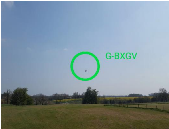
Screen shot in augmented reality mode showing identification of a UAS (a DJI Phantom 3) flying with RelmaTech DBM installed.
