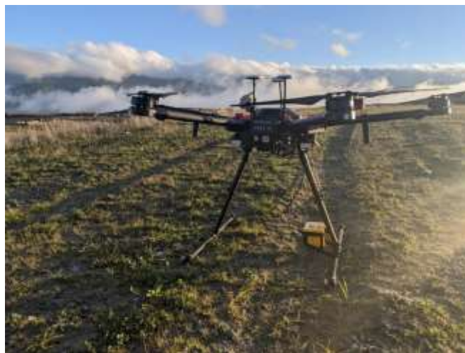
A UAV integrated with Falcon Laser Methane detector (c) Pergam
